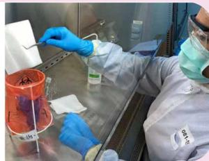
6 Wipe all BSC interior surface and all objects with a clothe filled with disinfectant, and the clothe will also be placed inside the BSC sterilized bag, and the bag will be sealed.
