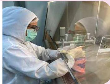
7 Shut BSC door and maintain its operation, and turn on the UV lamp for at least 30 minutes, then either resume work or turn off the BSC.
