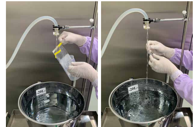
Figure 9: Monitoring personnel performs water system monitoring and sampling, using different pipe fittings according to other water quality sampling points.
